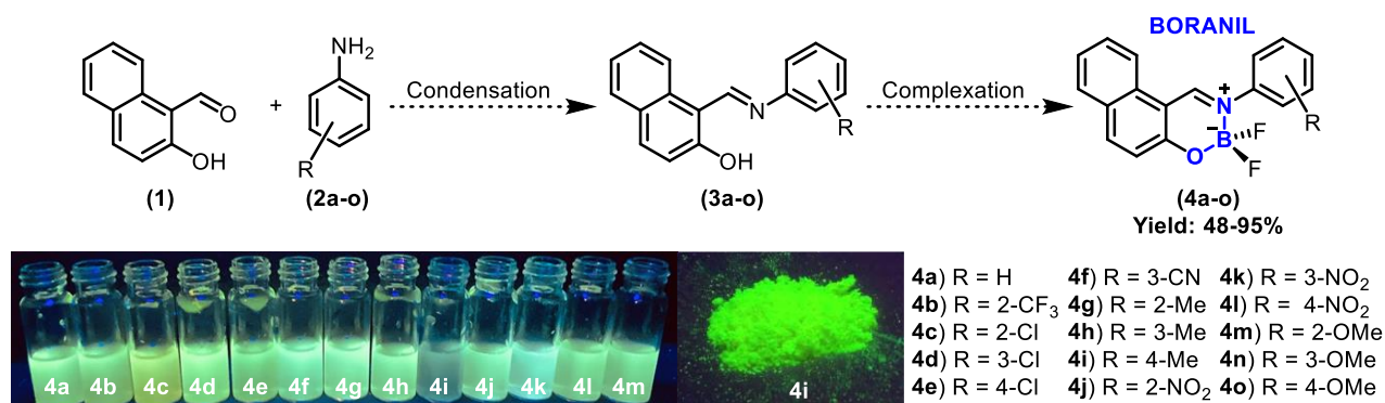
Scheme 1: Synthesis for obtaining the new fluorophores BORANIL ( 4a-o ). Compounds under the UV lamp (365 nm) in acetonitrile solution.
